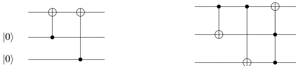
Figure 3: Encoding (left) and decoding (right) circuits for the three-qubit (bit flip) code.
